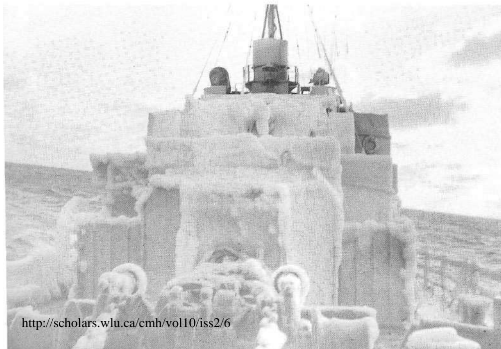
Photo 11: Icing, view from the bow. Months of winter weather and freezing spray frequently hampered ship's operations. The twin 4-inch guns, barely discernible below the funnel, are completely iced over. If ice build-up made a ship too top-heavy, it ran the risk of capsizing. Ice was always thicker on the side of the ship getting the most spray and, when conditions became dangerous, the captain ordered "all hands on deck" and the crew would chop away at the ice with axes.
