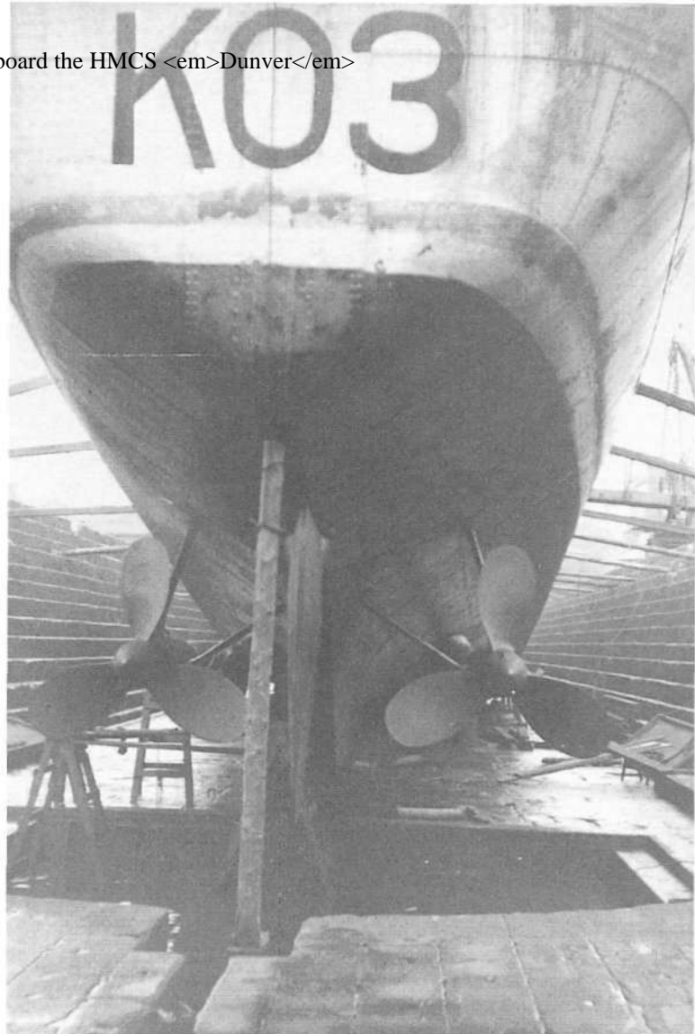
Photo 13: Dunver , pennant number K 03, in drydock at Pictou, Nova Scotia, stern view, late 1944. Frigates, originally designated 'Lengthened Twin-screw Corvettes,' were a much-improved design over the corvettes employed in the earlier years of the war. The frigates were larger, faster, more heavily armed, and had much greater endurance. Dunver's pennant number is unusually low and was made available by the transfer of HMS Heliotrope to the United States in 1942. 7 While all Canadian frigates were designated with the prefix K, none but Dunver used a two-digit pennant number.
